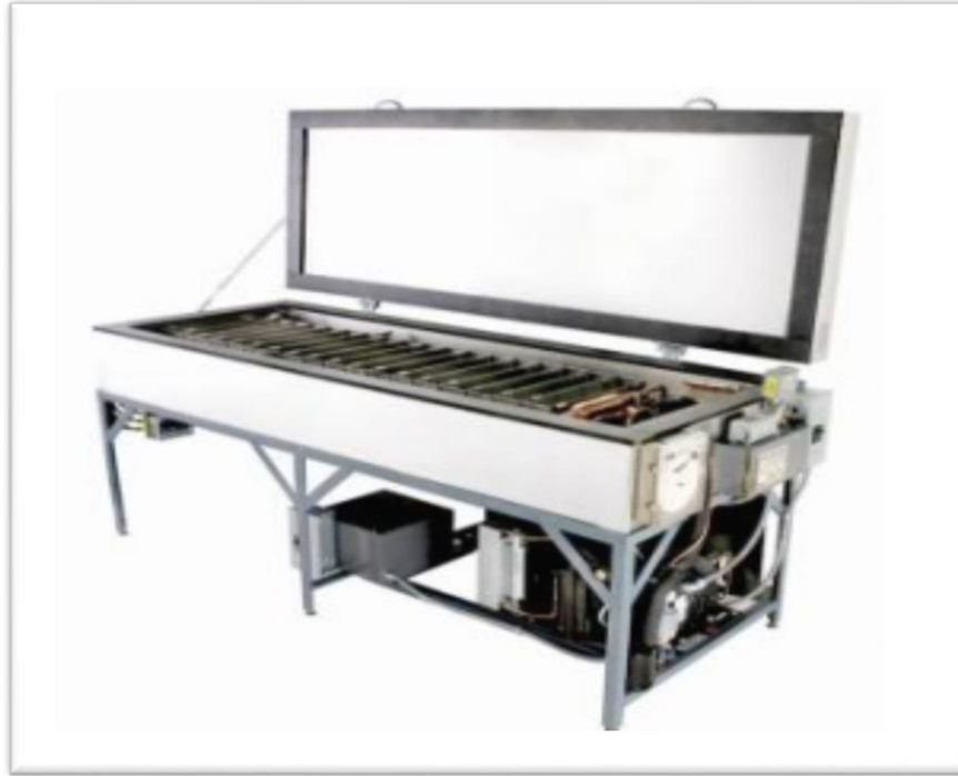
Figure 2.2: Gilson HM-120 Automatic Freeze Thaw Apparatus [3]
