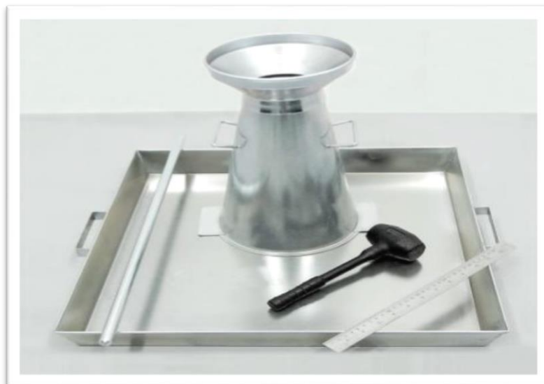
Figure 2.3: Material Set for Slump Test [4]
